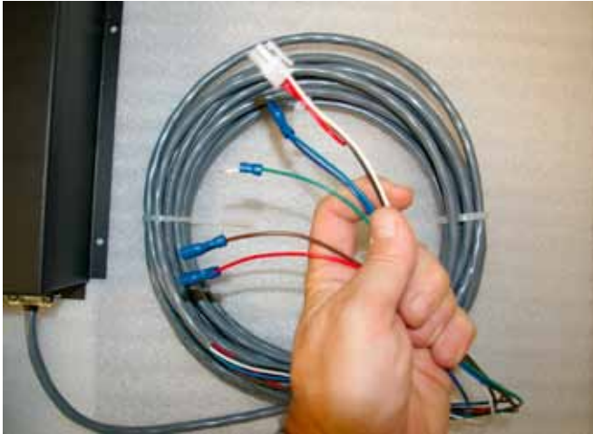
Figure 19. (Fireplace to Control Panel Harness)
